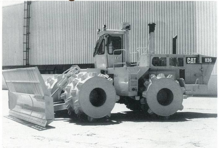
Caterpillar's Model 836 sanitary landfill compactor, the largest in their 800 Series of compactors.
